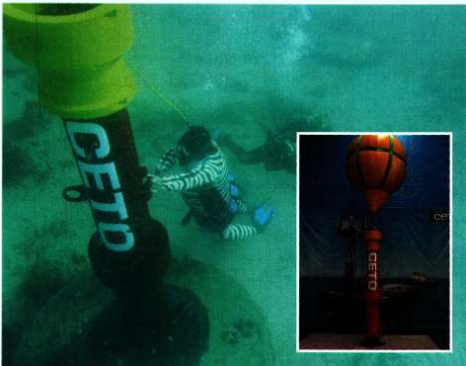
CETO is a new technology that converts ocean waves into energy and fresh water.
